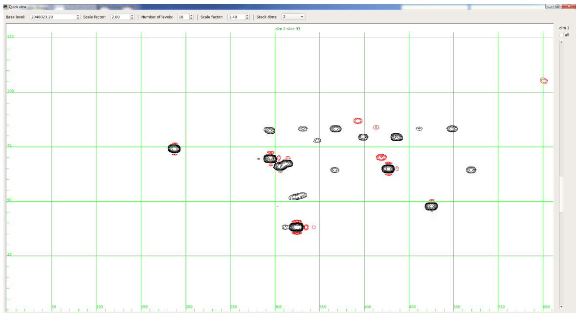
Figure 5.3: 3D spectrum display window for a single plane in the first indirect dimension (dimension 2, plane 37). 'All' (right-hand side) is now unticked and the slider used to scroll to the desired slice.
